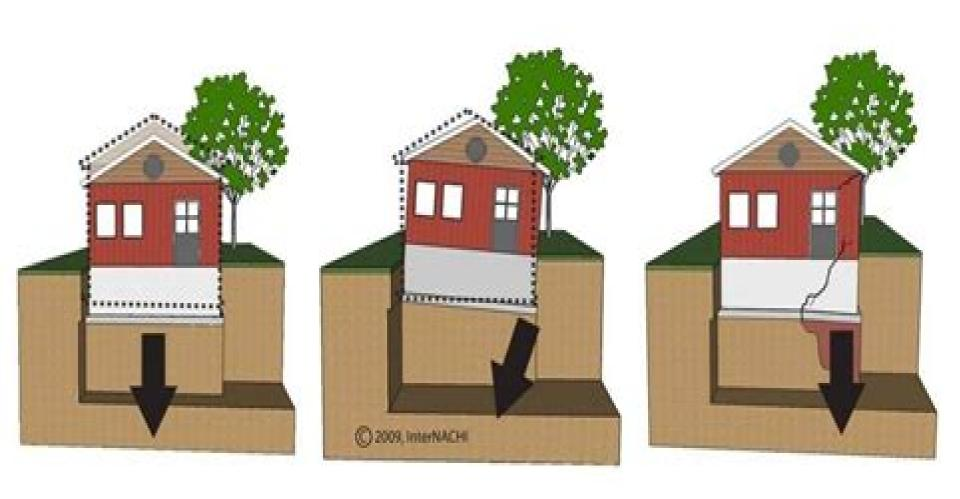
Uniform Settlement (No Cracks) Tipping Settlement (Mostly Without Cracks) Differential Settlement (With Cracks)
