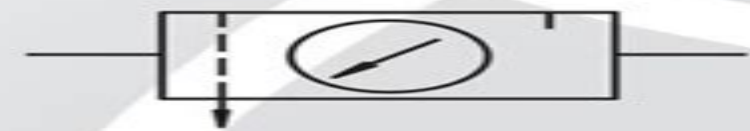
FRL with pressure gauge simplified
