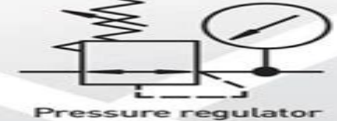
Pressure regulator with gauge
