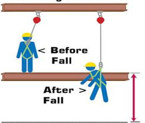
Illustration: Shock-Absorbing Lanyard With Cross-Arm Strap Anchorage Connector
