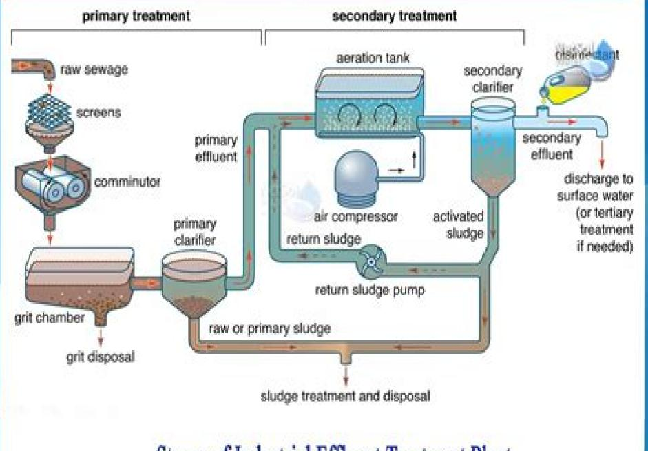
Stages of Industrial Effluent Treatment Plant
