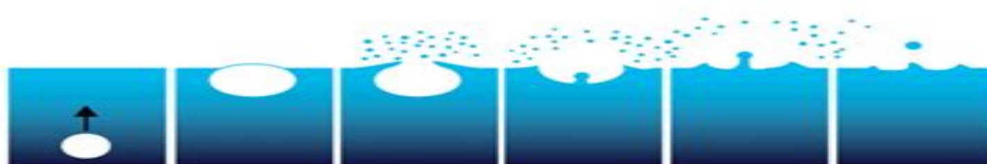
Mechanism of indirect sea salt aerosol production by bursting air bubbles.
