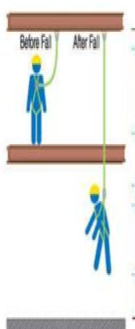
**Length of Anchorage Connector Length of Connecting Device** (Lanyard or Self-Retracting Lifeline) Required **Fall Clearance** Maximum Elongation/Deceleration Distance Harness Stretch/Sliding Back D-ring Movement 18 1/2 ft. (5.6 m) Height Measured to Worker's Harness Back D-ring Salety Factor
