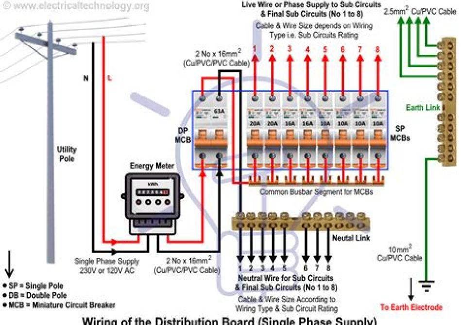
Wiring of the Distribution Board (Single Phase Supply) (From Utility Pole & Energy Meter to the Consumer Unit)
