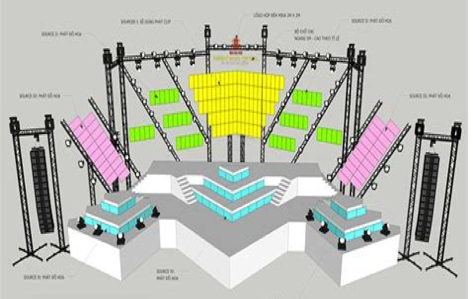
SÚ DUNG PS OUTDOOR - CABINNET 1000MM X 500MM CÁC SOURCE BÓ TRÍ THEO MÁU TRÊN BÁN VỀ. TÔNG CỘNG DÙNG 5 SOURCR BAO GÔM: 1 SOURCE TÔNG VÀ 4 SOURCE THEO 4 MÁU
