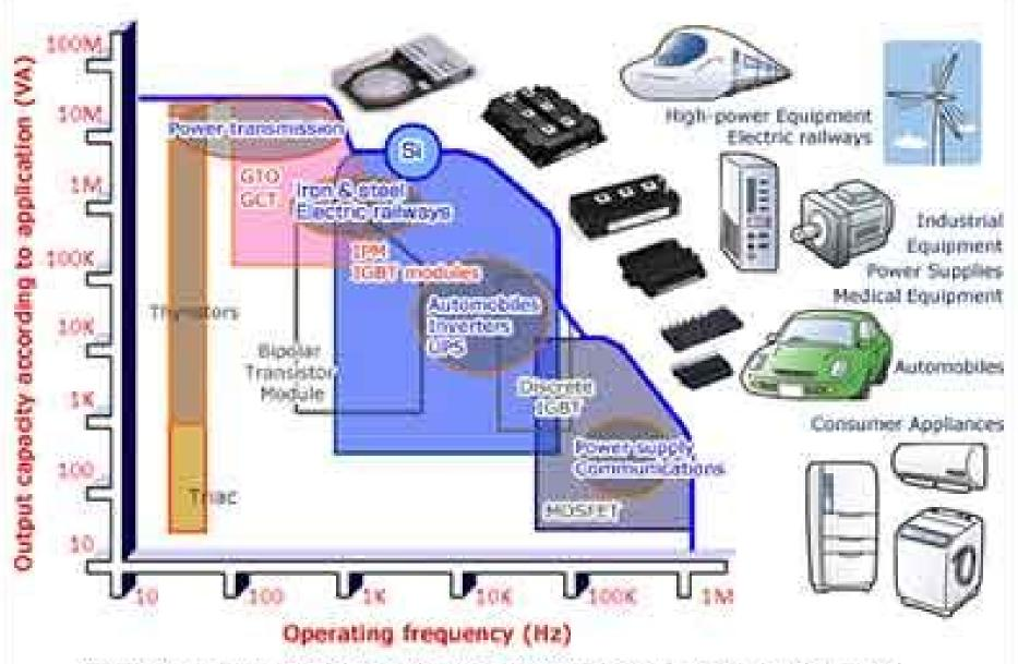
Currently, the majority of the development in power electronics applied in the area of mid- to high-power conversion is sustained by the evolving IGBT and IPM technologies.
