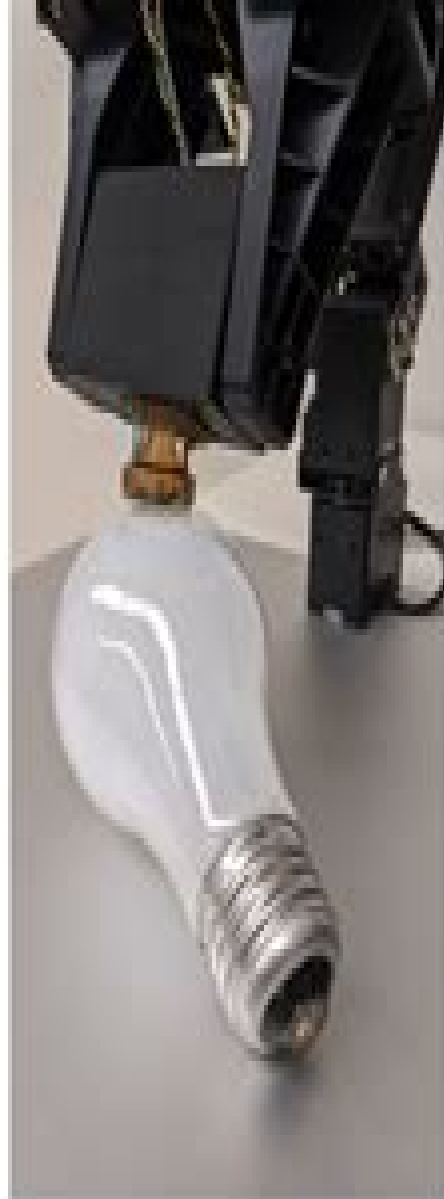
(b) Tactile module touching a object's surface.
