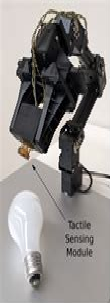
(a) Single tactile module on a robotic probe.
