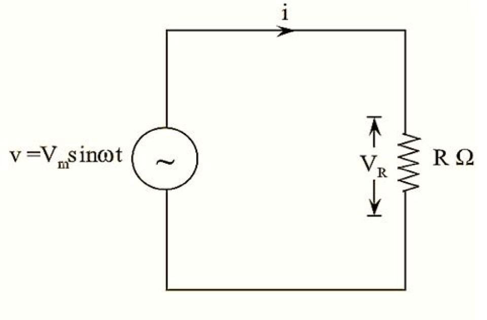
Figure (1): Pure Resistive Circuit
