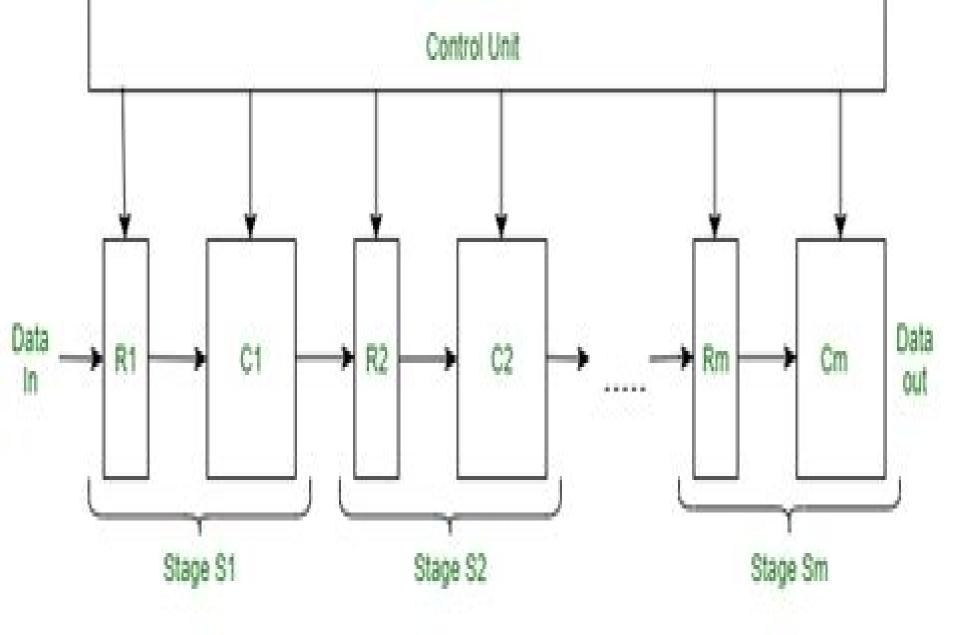
Figure - Structure of a Pipeline Processor
