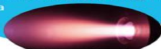
Fig. 1: Picture of IPG3 in operation. Mass flow rate of oxygen is 0.22 g/s at an anode power of 2.0 kW.
